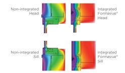
These thermographs prove that Formavue windows significantly increase thermal performance at the window wall interface compared to non-integrated windows.
